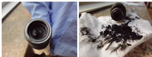
FIG. 4. Foulants at the reactor inlet during a hydrocracking pilot plant testing campaign.
